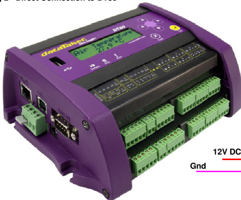
Fig 2 - Direct Connection to DT80
